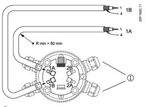
① For 1-path sensors exchange the two unused cable glands with the blind plugs.
