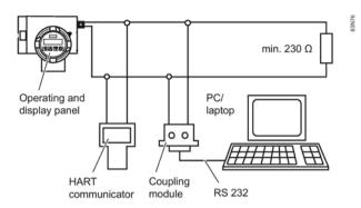
Figure 6-2 Operating via HART communication
