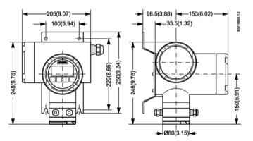
Figure 10-1 FUS060 with standard mounting bracket.
