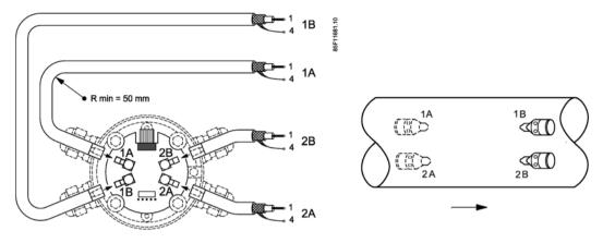
Figure 5-3 Wiring transducer cables, 2-path system
