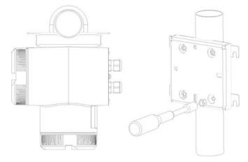
Pipe mounting with assembly bracket
