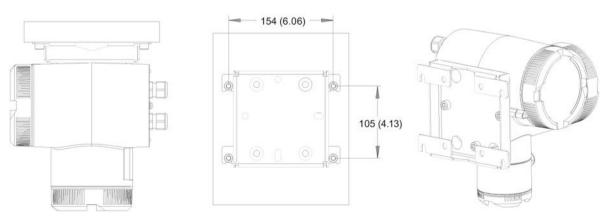
Wall mounting with assembly bracket. Dimensions in mm (inch).
