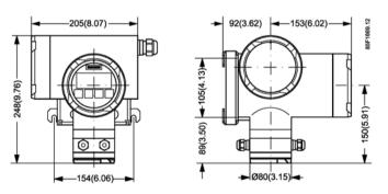
Figure 10-2 FUS060 with the optional special mounting bracket.
