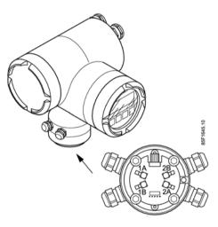
3. Carefully press the cables into the cable glands until the "snap" function fixes the cable inside the connection module. Make sure the cables are mounted correctly by smoothly pulling the cable.
