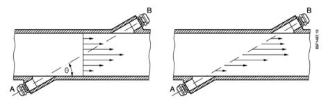
Figure 3-2 Velocity distribution along sound path
