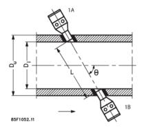
The ultrasonic signal is sent directly between the transducers. The advantage gained sending signals from point to point is an extremely good signal strength.
