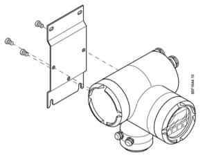
Figure 4-1 Standard mounting plate
